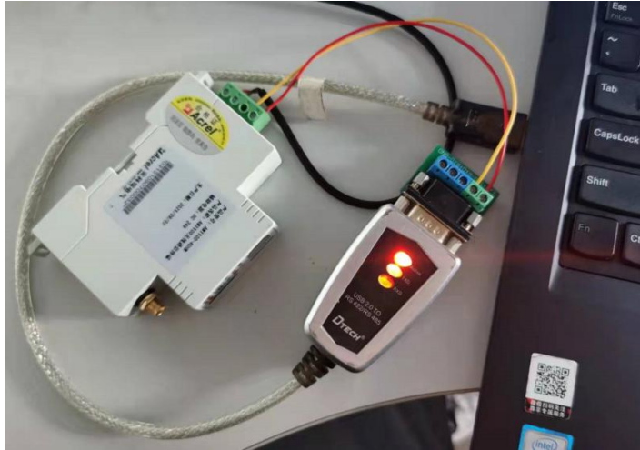
Wiring diagram of USB to 485 line
